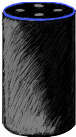
Figure 1: The Amazon Echo, a popular smart speaker. The Echo has four physical buttons on top (volume up, volume down, mute and action) and visual feedback is limited to an LED ring that can pulsate and change color [2].
