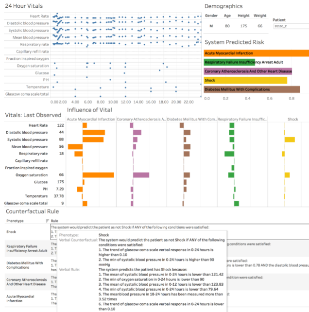
Figure 3. Screenshot of the AI-driven medical diagnosis tool with explanation sketches showing a patient with high predicted risk of acute myocardial infarction (AMI), heart disease, diabetes with complications, shock, etc. Explanations include (top left) feature value time series, (top right) class attribution of predicted disease risk, (middle right) feature attribution by vitals, and (bottom) counterfactual rules indicating key rules for each prediction. Interpretation: e.g., explanations suggest that the AI thinks that the patient has shock because of low oxygen saturation and blood pressure.
